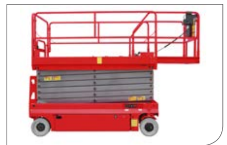
Larger working area thanks to the extendable platform
