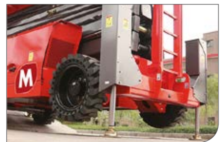
Hydraulic stabilisers with automatic levelling
