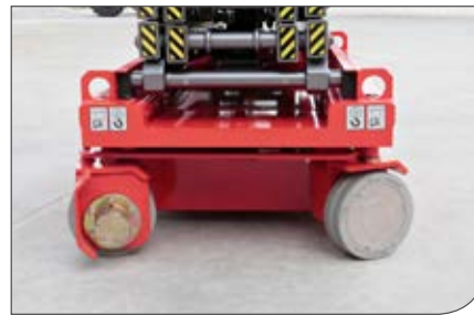
DC drive motors with steel covers providing zero turning radius
