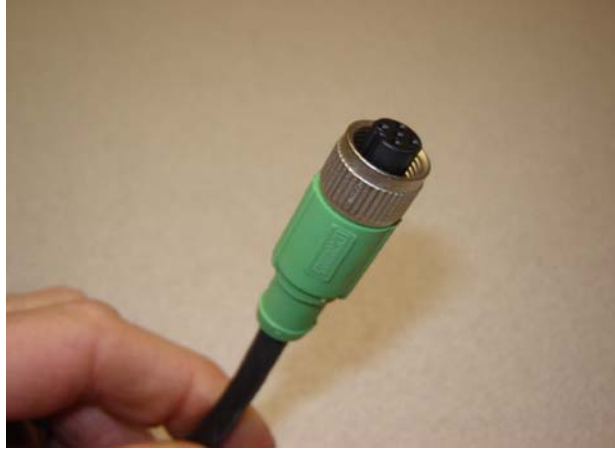
Figure 8-8. Phoenix Contact M12 – No Dielectric Grease
