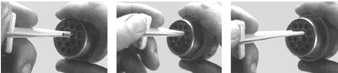
Figure 8-20. HD/HDP Contact Removal
