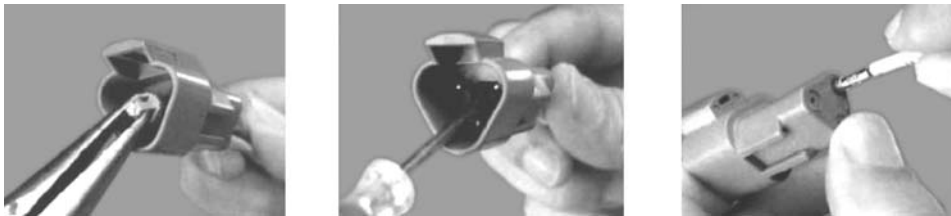
Figure 8-17. DT/DTP Contact Removal
