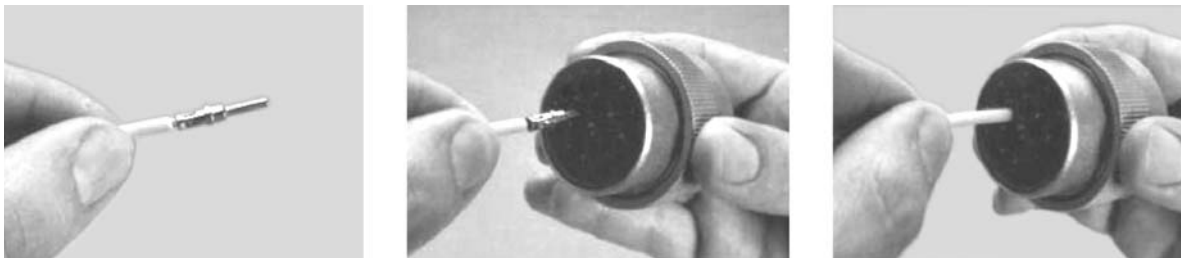
Figure 8-18. HD/HDP Contact Installation
