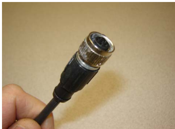
Figure 8-7. Brad-Harrison M12 – No Dielectric Grease
